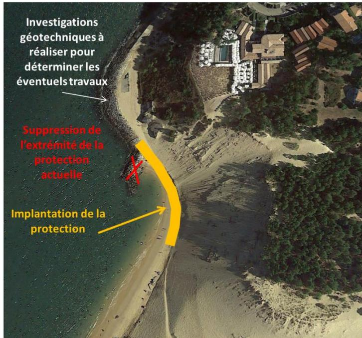
Figure 15 – Implantation de la protection
